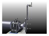
The Offset laser fixture is adjustable in a plane parallel to the flange face of the stationary machine and can be set at any position to eliminate the offset from the driven unit.
