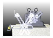
The Offset fixture comes with a number of methods of attachment. The system is designed so you can, in most cases, utilize the coupling bolts themselves when mounting the arm on the flange.
