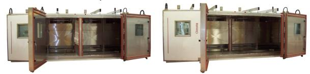
A supervisor connected to the two control PC enables to synchronize these two equipments in order to get a very good regulation within the temperature and humidity whole range.
