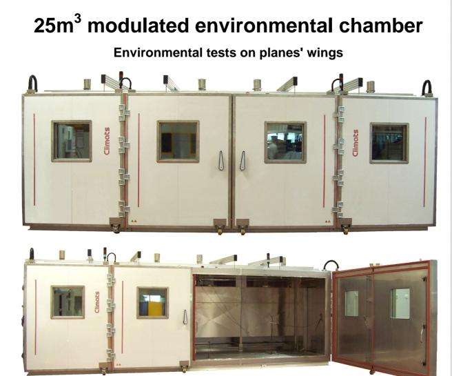
Two environmental chambers, at first totally independent in term of functioning, but that could be put together for tests on longer planes' wings.
