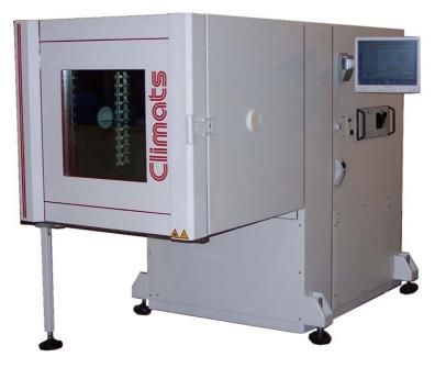
343 dm<sup>3</sup> climatic chamber, adaptable onto a shaker, with plate accessories to be used as a standard chamber.
