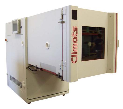
512 dm<sup>3</sup> environmental chamber designed to be adapted on a vibrating pot.
