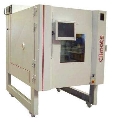
1130 dm<sup>3</sup> environmental chamber designed to border a concrete foundation in order to realize thermal tests with a perfect vibratory stability.
