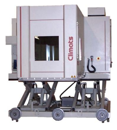
Hot-Cold-Humid Rapid Temperature Cycling type of climatic chamber (1200 dm<sup>3</sup>) set on a lifting table intended for combined temperature / vibrations tests.
