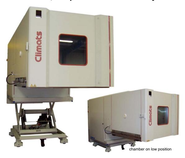
Set on two 5 m long rails perfectly aligned, this chamber – meant for electronics area – can still move on two axes in order to easily free the working space for the tests preparation.
