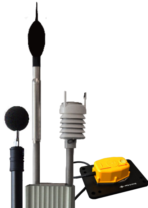
EMU includes simultaneous weather, vibration, Class 1 audio and blast - all in one.
