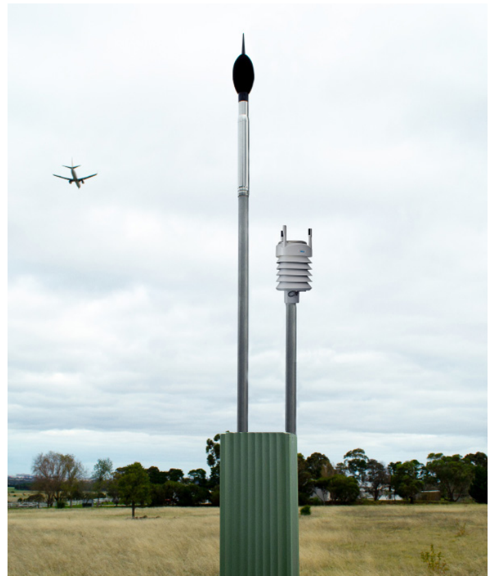
EMU set-up on site with Microphone and Weatherstation
